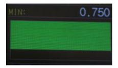
TM281 series thickness gauge has time base B-scan function. Move the probe along the workpiece surface, then the cross -sectional profile of the workpiece display, use for observe the underside contour of the workpiece. It could be automatically capture a minimum value of the B-scan image, and indicate the position of the minimum by a red triangle. You can see any point thickness value of the B-scan image by moving the pointer.
