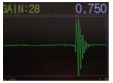
Users could directly see the color waveform of the ultrasonic sound (or A-scan) on the screen, which is quite important for the occasions that we need to check the correctness of the testing results. Many cases will cause wrong testing results or even noreadings. We could find the causes easily through the A-scan. Adjust the three parameters of GAIN, BLACKING, GATE, and then we will get the right readings.
