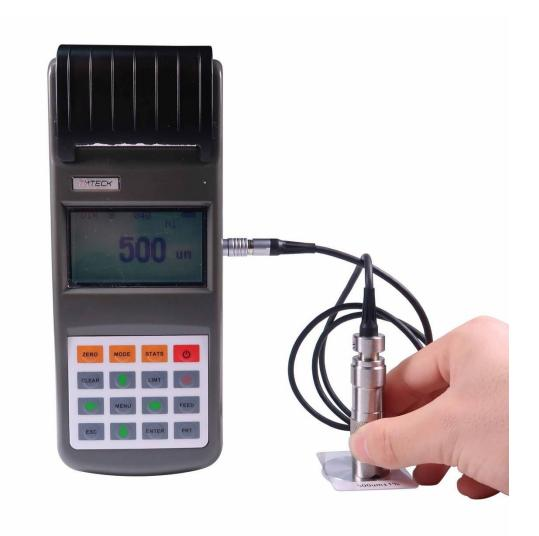
Portable Digital Coating Thickness Gauge TM260 adopts two thickness-measuring methods: magnetic induction (ferrous) and eddy current (non-ferrous). It can rapidly, nondestructively, and precisely measure the thickness of non-magnetic coating on magnetic metal substrate, and the thickness of non-conductive coating on non-magnetic metal substrate. This paint meter can be equipped with 6 optional probes for different applications. It is suitable for both field testing and laboratory research.
