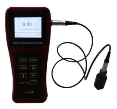
TMD-102 is a kind of eddy current electrical conductivity meter, which is designed f or quick & convenient measurement of material property, such as material separate, quality control, material state check and so on. It uses the electromagnetism testing principle. Testing objects focus on non-ferromagnetic material.
