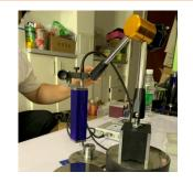
TA1420-Magnetic flexible base for simple test ,easy move and comfortable using
