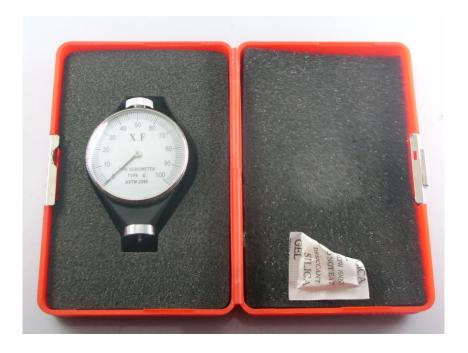
**TS-OO** durometer is an essential characteristic of Rubber foam, sponge, plastic foam, silicone, gelatinous materials, textiles, low-density coils. products. It is feature portability, ease of operation, with facility, high resolution and it is available in GB/T 531 -1999 and ISO 7619, ASTM D2240.
