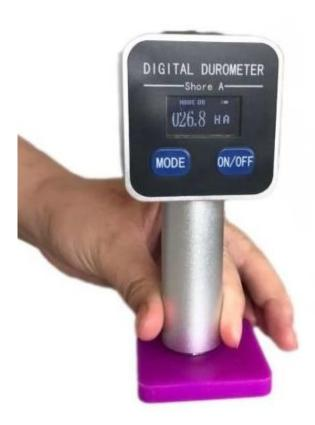
NEW TYPE digital shore durometer, rubber hardness tester, shore hardness tester TS-300(TS-300A and TS-300D)
