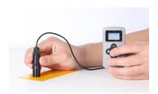
NFe-based probe detects the thickness of all insulating coatings sprayed on non-magnetic metal substrates (such as aluminum, copper, brass, stainless steel, etc.), such as paint layers, powder coatings, ceramic coatings, etc.
