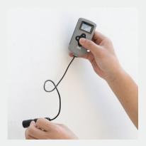
5. The coating thickness gauge has basic mode, quality control mode, continuous mode and statistical mode to choose from, adapting to more test scenarios
